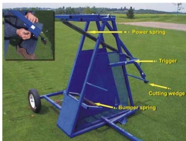
Figure 1. Divot making machine. Inset shows adjustment of the variable depth cutting wedge.
